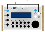
Press the rightmost white button and hold it down while you turn on the unit with the blue power switch on the left. This tells the unit "we are ready to update the firmware". The display will read as shown below.
