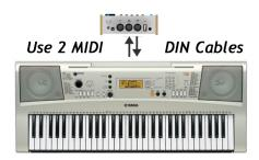
In the above diagram, MIDI OUT from the source is connected to MIDI IN on TBX2b, and MIDI OUT from TBX2b is connected back to to MIDI IN on the source, which is also the destination. TBX2b sends *Local Control OFF* to disconnect the source from the destination. If *Local Control* is not turned OFF, two notes will sound for every key pressed.
