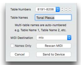
TBX2b assigns one tuning table per MIDI channel, with 128 notes per tuning table, so if your tuning contains more than 128 notes, it will be broken into multiple tables in TBX2b memory. For example, Tonal Plexus tunings contain 2048 notes (16 x 128 = 2048), so the tuning is spread across 16 tuning tables in TBX2b memory. UTE figures out how many TBX2b tuning tables
